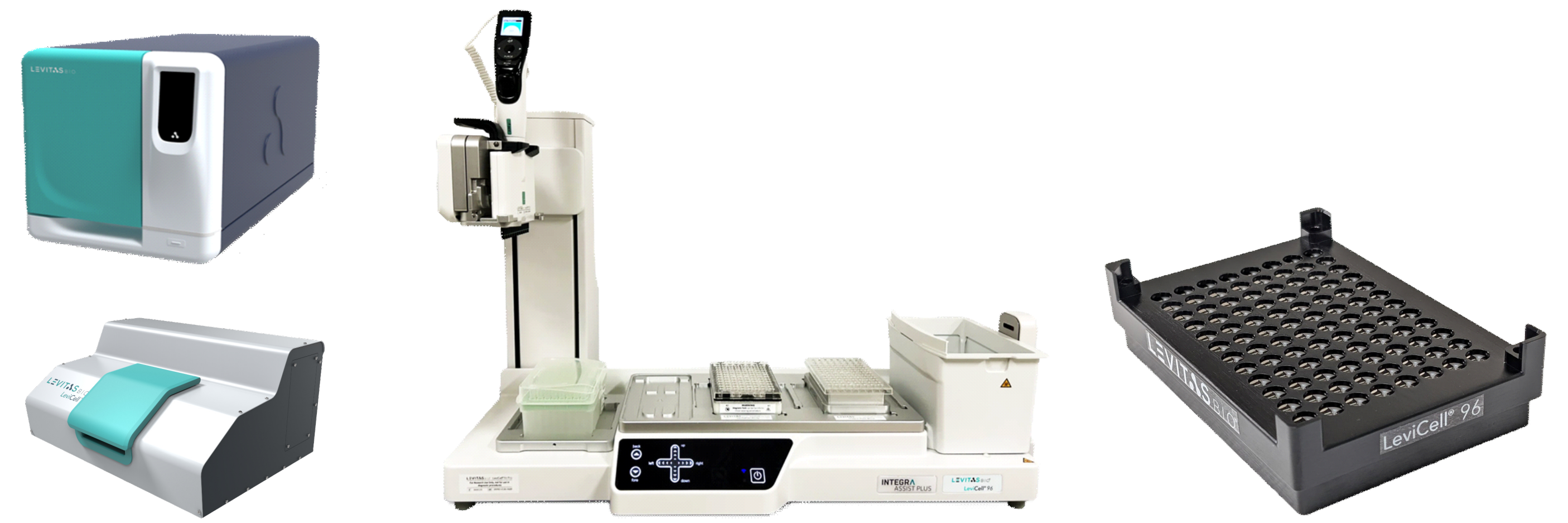
Figure 1. The LeviCell enrichment technologies - LeviCell 96, center; LeviCell EOS, top-left; LeviCell 1.0, bottom-left; and the Selective Arrayed Levitation Technology array (SALT), right. The magnet arrangement of the SALT allows for 96 simultaneous levitation reactions. The cartridge based systems can provide either 4 sample processing (LeviCell EOS) or single sample (LeviCell 1.0) enrichment.
