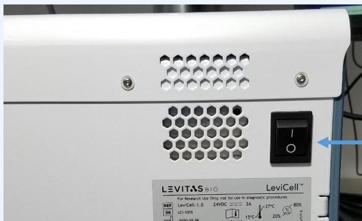
Figure 4. Instrument power switch, shown in the OFF “O” position. Leave it OFF (“O”) until instructed.
