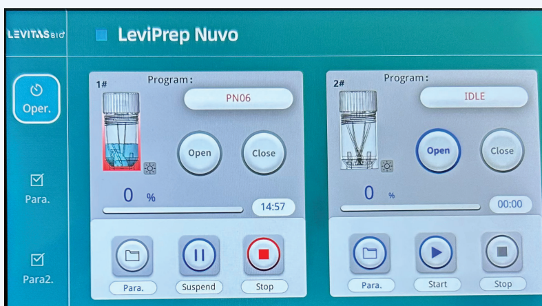
Figure 4. Operation Interface elements. This figure shows an overview of the key interface components, including main menu, program indicators, sample tray controls, and temperature status indicators.
