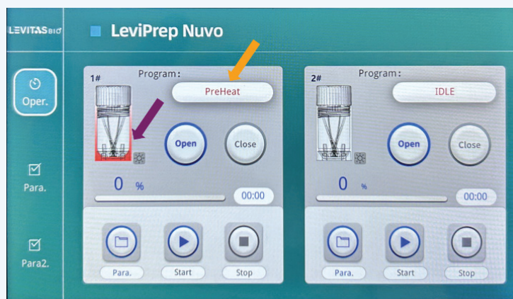
Figure 14: Operation Interface during preheating
