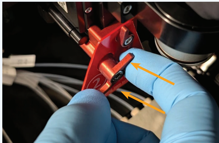
Figure 11. LeviCell EOS focus stage safety lock larger thumbscrew.
