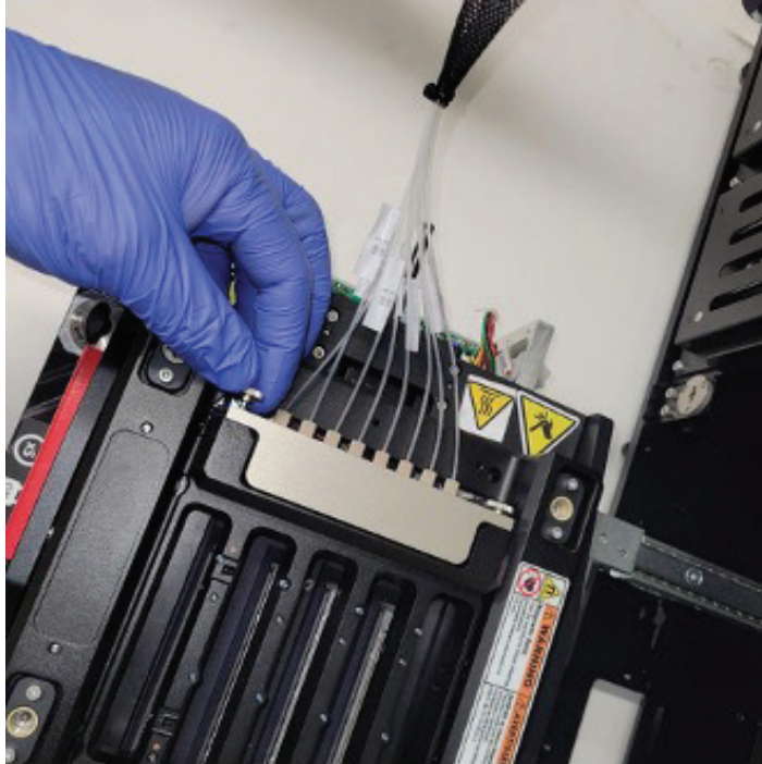
Figure 103. Core module top view and manifold thumbscrews
