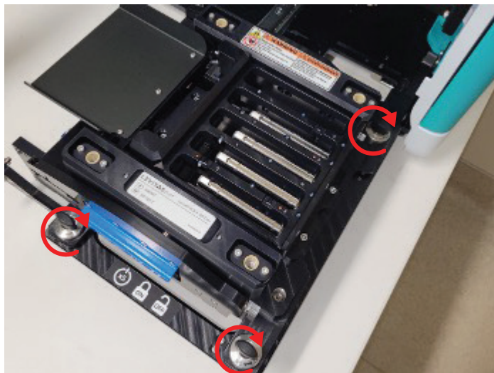
Figure 110. Switch the three Core module locks into the cradle to ON
