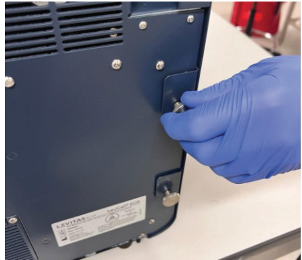
Figure 117. Rear side panel thumbscrews
