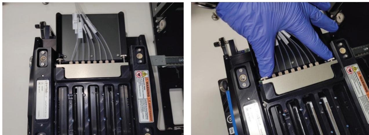
Figure 112. Fastening the pneumatic manifold block onto the core.
