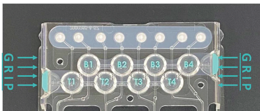
Figure 1: EOS-4 outlet wells and gripping points
